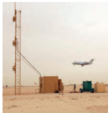
The Thales Deployable Instrument Landing System is for unimproved airports, or those with damaged facilities.
